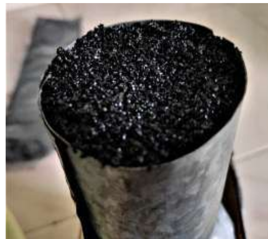
Figure 6.6 Module stuffed with GAC
