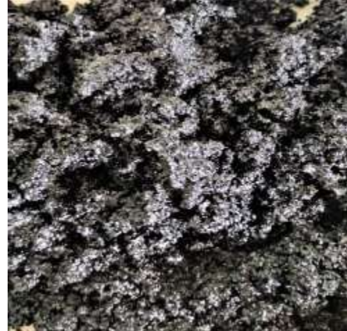
Figure 6.5 activated carbon blended with epoxy
